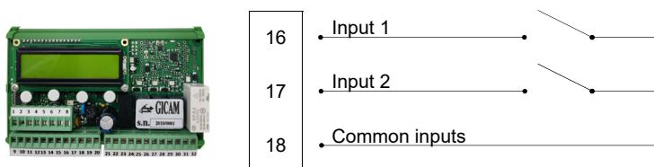
**Attention:** If the appropriate function is selected on the inputs, the blocking threshold has two values (A and B). the instrument uses threshold values A or B depending on the status of the inputs.
